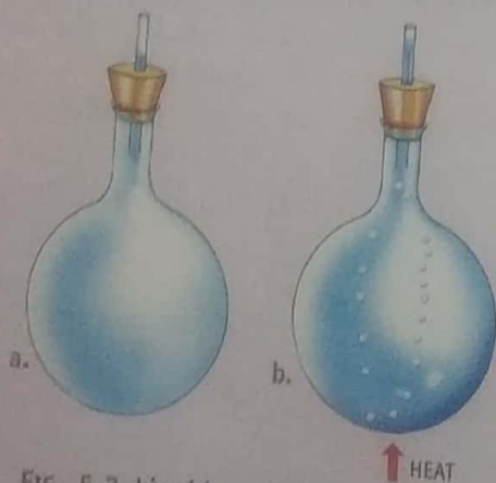
FIG. 5.3 Liquid expands on heating.
