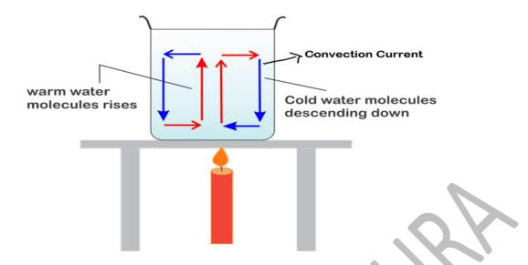
Consider the above figure that shows heating of water in a pot. Here in this process, all three modes of heat transfer can be seen.
