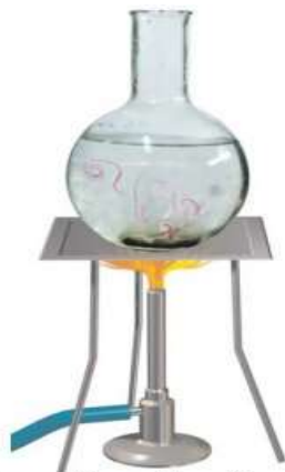
Convection of heat in water
