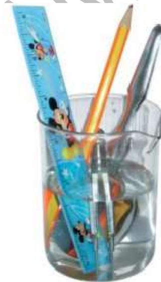
Conduction of heat by different materials
