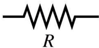
(a) symbol of a resistor (b) Colour coded carbon resistors
