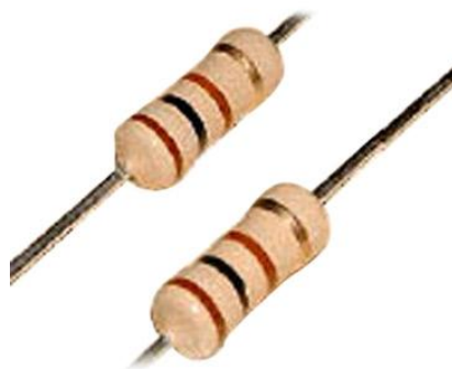
(a) symbol of a resistor (b) Colour coded carbon resistors
