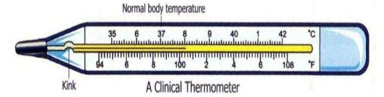
\*Mercury is a toxic substance and is very difficult to dispose off if a thermometer breaks.
