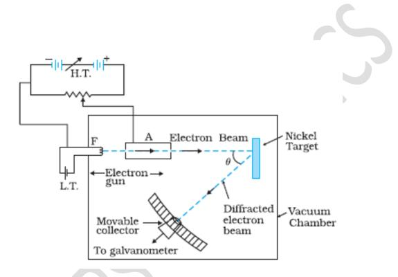
The experimental setup consists of an electron gun, which comprises of a tungsten filament coated with barium oxide and heated by a lowtension battery.
